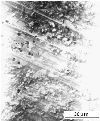
Figure 10 Wear tract of tested metal matrix composites.
